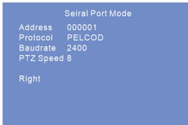
Note: In serial port mode, many PTZ operations can be done, such as change direction, zoom in/out, adjust IRIS, call or set preset, etc.
